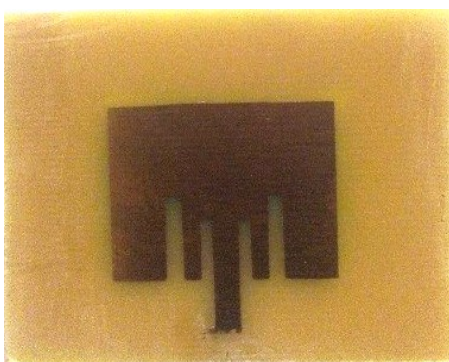
Figure 6b: Fabricated optimized antenna
